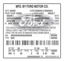
**GVWR (Gross Vehicle Weight Rating)** – is the maximum allowable weight of the fully loaded vehicle (including all options, equipment, passengers and cargo). **The GVWR is shown on the Safety Compliance Certification Label located on the B-Pillar or the edge of the driver's door. The GVW must never exceed the GVWR.**
